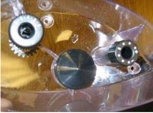
Step 9: Before placing the Bean Hopper back onto the machine you must make sure the adjuster knobs are in the correct positions. Put the grinder adjustment knob to 6 and the doser knob to the plus ( + ) symbol.
