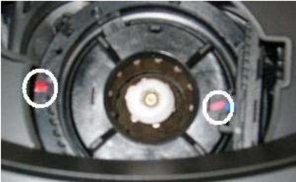
**Step 2:** Remove the Rubber Gasket on top of the Grinder. Once removed, rotate the outer ring counter-clockwise until the red lines are opposite from one another. The outer ring should not be able to rotate any further.
