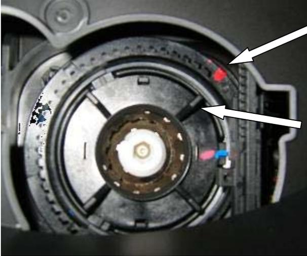
Step 6: Rotate the outer ring Clockwise until the red line is aligned as shown below with the fin on top of the burr.
