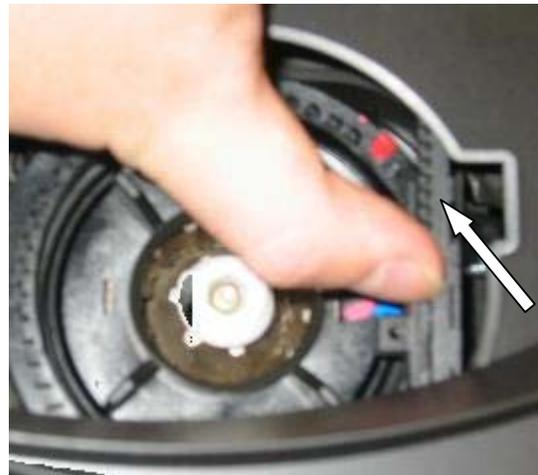
Step 8: Replace the rubber gasket onto the top of the upper burr.
