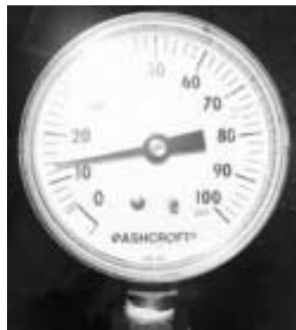
FIGURE 5. Low Water Volume = less than 25 psig
