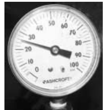
FIGURE 6. Proper Water Pressure Volume = greater than 25 psig
