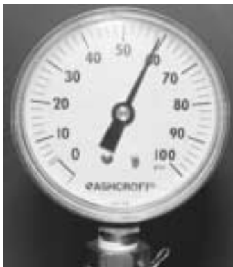
FIGURE 4. Static Pressure = 60 psig
